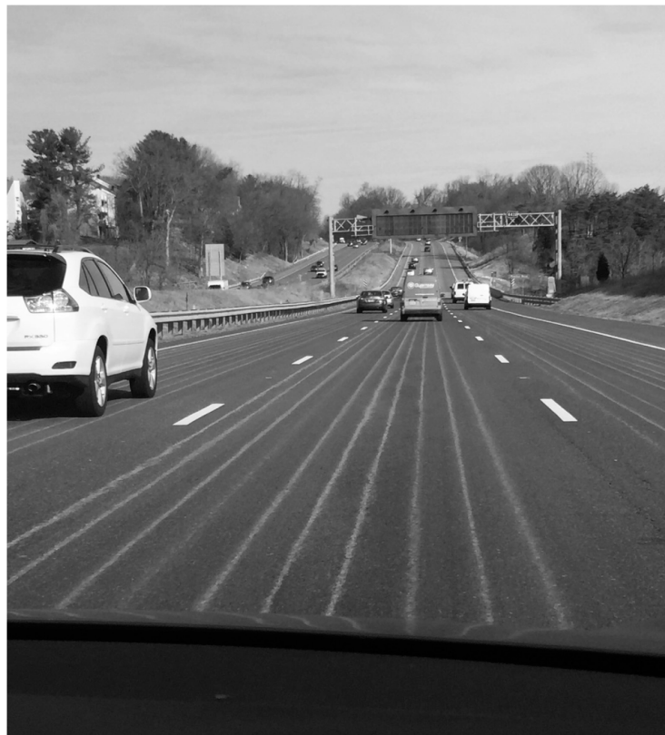
FIGURE 14: Salt lines on a highway, in advance of a forecasted snowstorm, were reported to be confusing Tesla's Autopilot feature.
